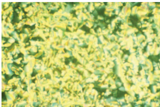
Figure 5. Fan texture of the hexagonal columnar phase exhibited by the tetracatenar oxadiazole ( 8 ; R_1=R_2=C_{12}H_{25}O ; R_3=H ).
