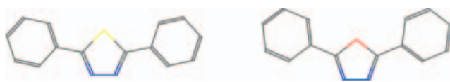
Figure 9. Comparison of the structures of thiadiazole (left) and oxadiazole compounds as modelled using Chem3D Pro software. The internal C-S-C bond angle is \sim 148^{\circ} for the thiadiazole and the internal C-O-C bond angle is \sim 127^{\circ} for the oxadiazole.
