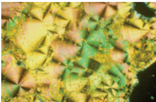
Figure 7. Circular domain texture exhibited by the tetracatenar oxadiazole ( 9 ; R_1=R_2=C_8H_{17}O ; R_3=H ).
